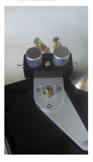
15. Install the adjustable tonearm base and tonearm, connecting the Lemo plug into the top of the Bob's Devices SUT box.
