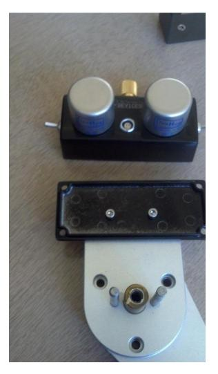
10. From the underside, install the provided 4 Phillips head screws to attach the Bob's Devices base plate to the SUT and ensure that they are snug.
