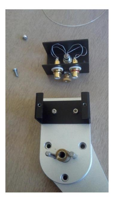
6. Remove the Allen head screw holding the control box base to the tonearm base plate. You will reuse these screws to attach the Bob's Devices SUT base plate.
