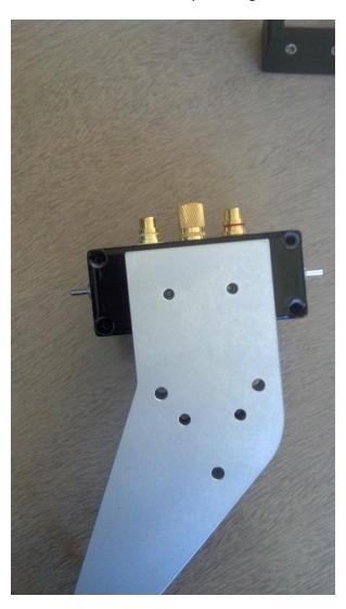
11. The top should fit snugly and not be loose. Don't be afraid of over tightening these screws. Use a # 2 Philips head screwdriver.
