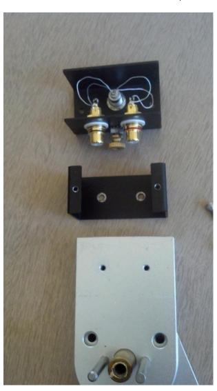
7. Attach the Bob's Devices SUT base plate to the VPI tonearm base using the screws just removed.
